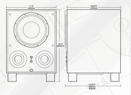
Note: Depth dimensions exclude front knobs and rear speaker connectors. Add 1 1/2" plus required wire spacing. Frequency Range (-6dB):
