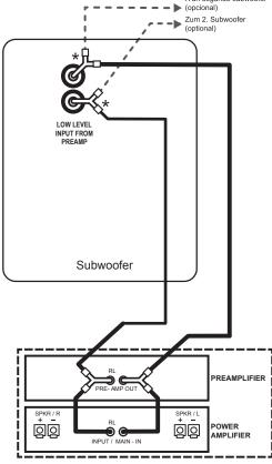
ALTERNATE: RECEIVER OR INTEGRATED AMPLIFIER WITH PRE-AMP OUT AND MAIN-IN JACKS
