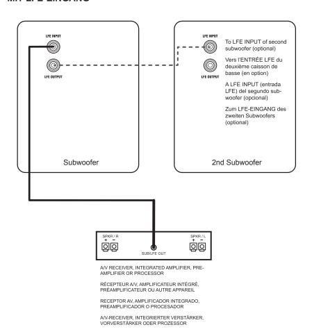
Use this configuration to connect the subwoofer to an A/V receiver or processor's subwoofer/LFE output provided your A/V receiver/processor subwoofer/LFE output is low pass filtered.
