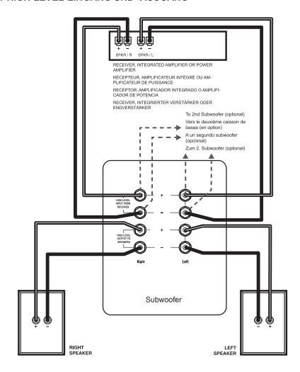
High level connections wire the subwoofer to the speaker output terminals of a receiver or amplifier, just as if the subwoofer was a pair of speakers.
