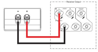
**Observe Proper Connection Polarity**
